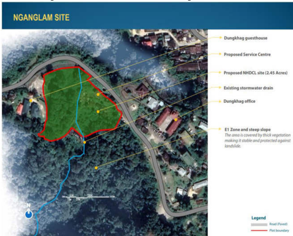
Figure 8: Natural Storm Water Canal/Drainage at the Site
